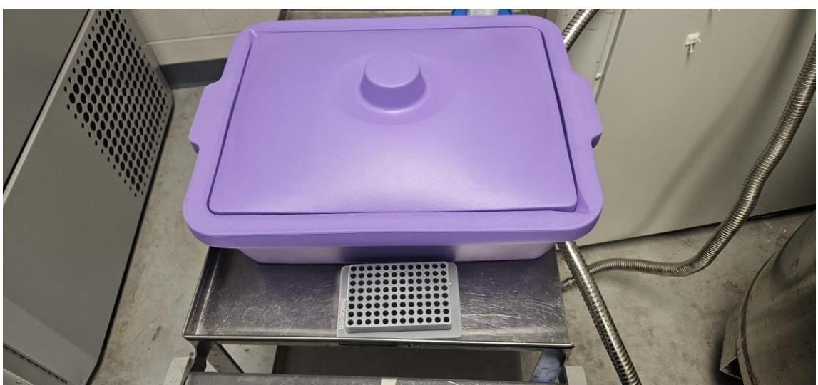
This is an example of an LN2 transfer pan using smaller cool cell racks and a Cole-Parmer EVA Ice pan and an insulated dewar for transferring LN2 from a 22PSI tank.
